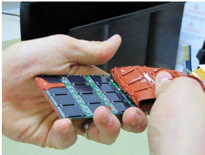
Figure 20: Removal of internal protective layers
