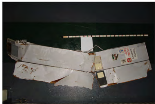
Figure 37: Metallic stiffeners deformed by buckling
