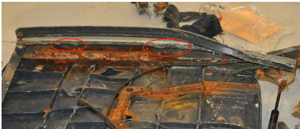
Figure 80: Roller marks on the guidance rail
