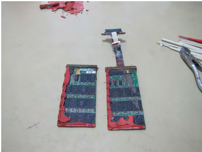
Figure 23: CVR memory boards before cleaning
