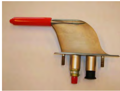
Figure 3: Pitot probe (with protection caps)
