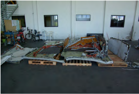
Figure 38: Floor of the LDMCR: with bottom-upwards deformation
