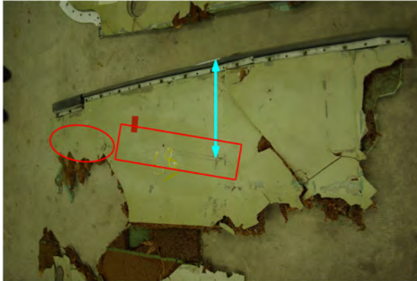
Figure 43: Part of the No. 3 flap track fairing on the left wing
